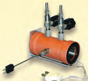
Figure 2 Gas cell configuration with Swagelok® valves
