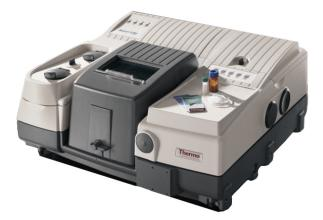
Infrared spectroscopy has been a workhorse technique for scientific analysis in the laboratory for over sixty years. As modern FTIR spectrometers have become more powerful, rugged, and reliable, their use has further migrated into the factory and into the field as well. For all manner of testing where the chemical (and occasionally biological) constituency of a sample or mixture is wanted, the FTIR is playing an increasingly important role. For example:
