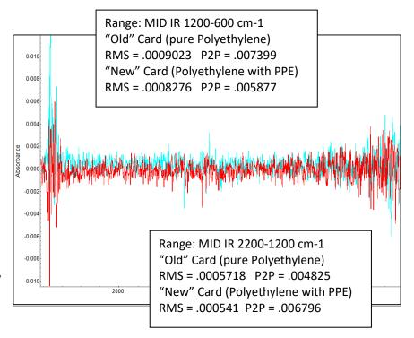
In the above example, the "old" card and the "new" cards are seen in the infrared, at 32 scans, 2cm-1 res., background vs. empty sample in absorbance. We measured the PeakToPeak noise and the RMS noise in the Near IR and Mid IR for comparison. We find only that while there is a small increase in Peak-to-Peak noise from the PPE in the new cards, the overall effect throughout the mid-IR range when measured as RMS noise in less remarkable.
