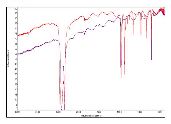
Above in Blue is the infrared spectrum of so called "Pure" Polyethylene substrate (approx. 16 microns thickness) alongside the newer material in Red which is Polyethylene plus Polypropylene, and which noticeably obscures the infrared spectrum with additional lines. Notice the prevalence of more mid-IR bands in the Red spectrum compared to the somewhat cleaner Blue spectrum derived from previous lots of Polyethylene IR cards.
