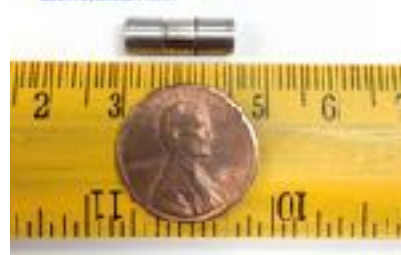
647nm Isolator Miniature optical isolators based on CdMnTe crystals as Faraday rotators for lasers in the region 630-850nm Isolator Dimensions: 1mm diameter, 15mm thickness Crystal Dimensions: 1.7mm x 1.7mm x 1.7mm Polarizer: Cube type 2.0mm x 2.0mm x 2.0mm Transmission: 78-79% Extinction Ratio: 30 dB or higher Beam Diameter: 1mm
